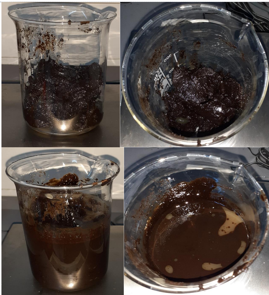
Figure 2: Wax, asphaltene, resin of deposits (WARD) emulsions formed.
